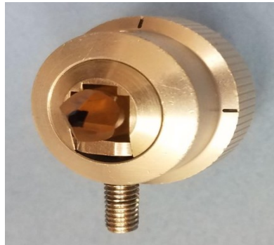
Block holder with Epon block mounted
